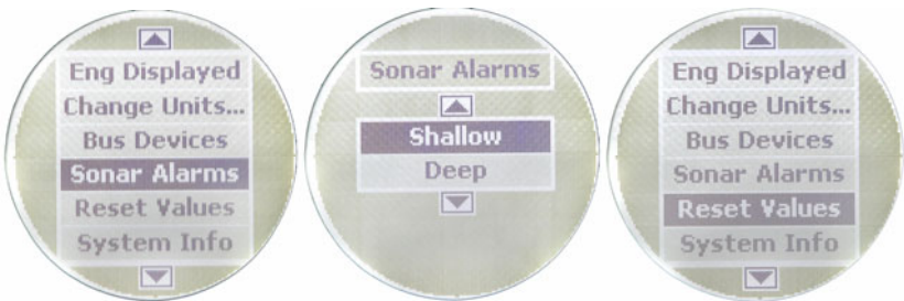
Sonar Alarms highlighted on System Setup menu (left). Sonar Alarms menu (center); Reset Values selected on System Setup menu (right).
