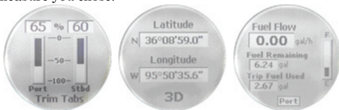
Trim Tabs page (left), GPS Module page (center) and Fuel Manager Page (right).
