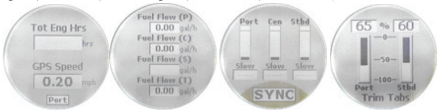
Dual Digital (from left to right), Quad Digital, Synchronizer and Trim Tabs page.
