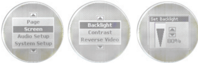
Basic menu with Screen highlighted (left). Screen option menu (center) with Set Backlight window (right).
